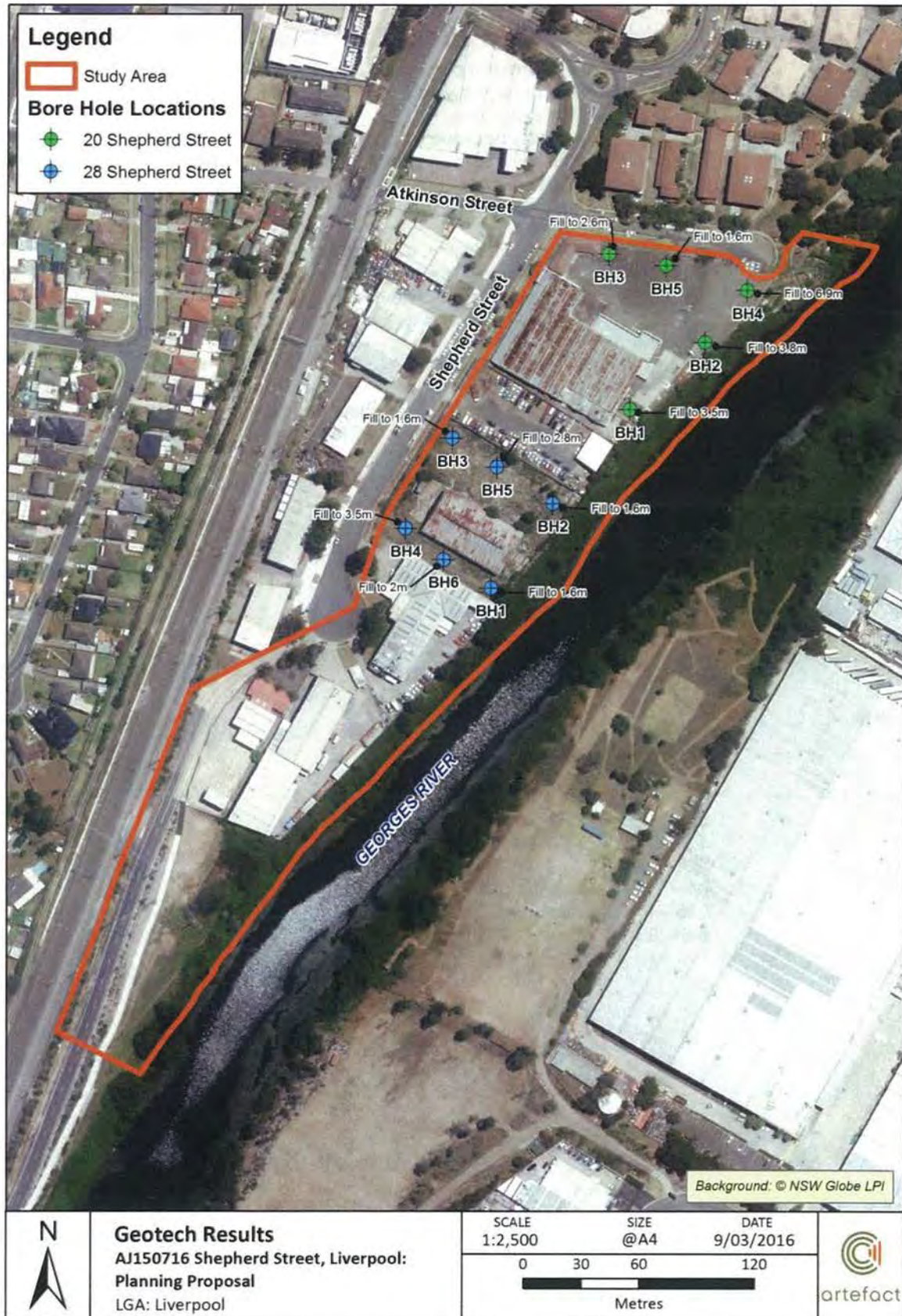
Figure 13: Location of geotechnical survey
